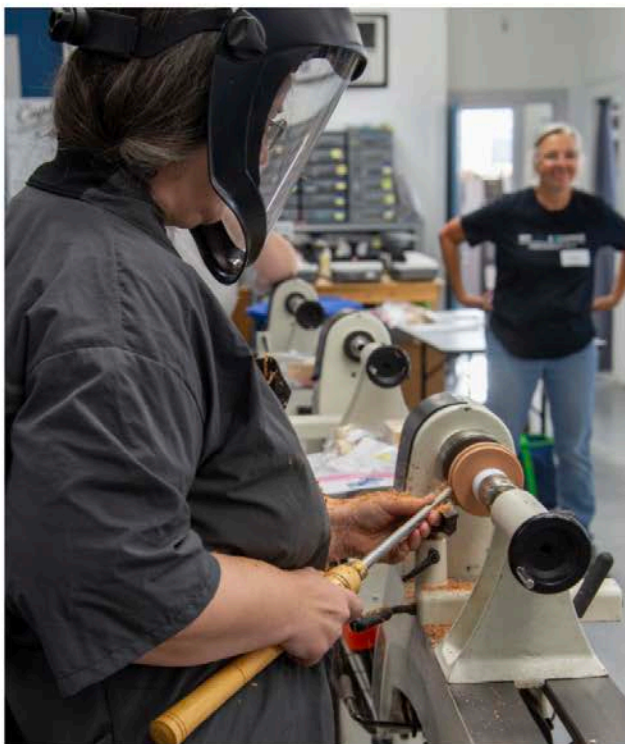
The class after a successful workshop! (top) Gretchen turns the rough profile of the bangle (left), and parts the bangle from the remaining pendant blank (above).
